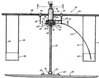
This is the drawing of the invention described in a patent entitled "Occupant-Propelled Roundabout Swing Set". A rider sitting in one of the swings can pull on a cable which causes the swings to rotate around the poll.
